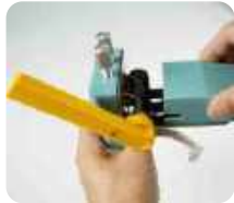
1. Loosen the screws, remove the lid.
